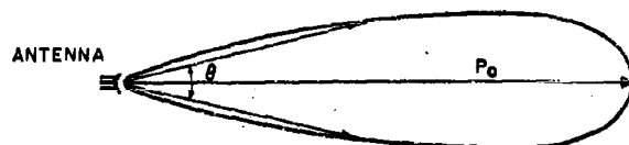
FIGURE 1. Idealized pattern of a microwave search radar. Length of radius vector is proportional to power radiated in that direction.
